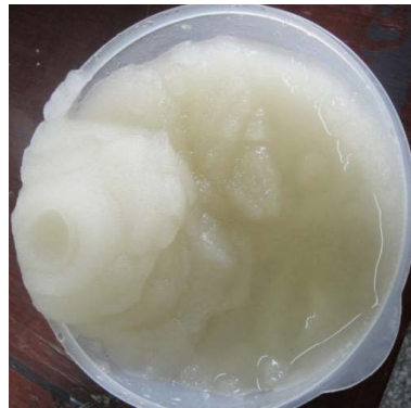
Figure 3. The physical figure of ice slurry made up by experimental methods.
