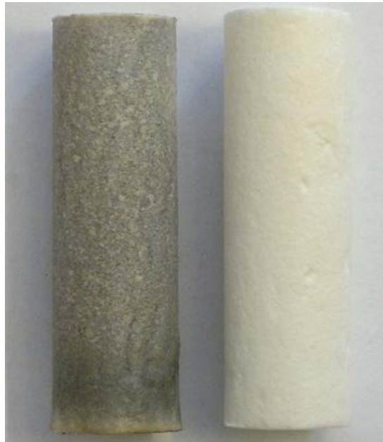
Figure 6. Filter with and without carbon particles.
