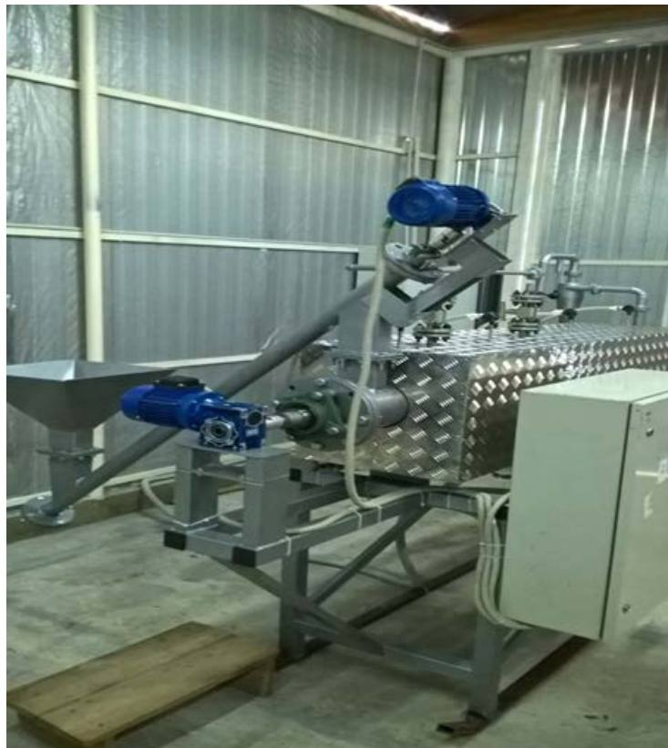
Figure 13. A pyrolysis reactor for solid biomass.
