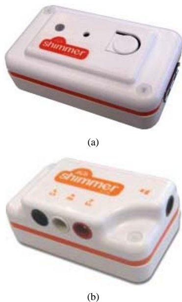
Figure 2. (a) Wireless 9 DoF sensor by SHIMMER; (b) Wireless wearable ECG sensor by SHIMMER.
