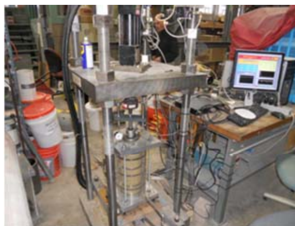
Figure 2. Triaxial apparatus for cyclic loading—University of Madison (Bâ, 2012 [10]).
