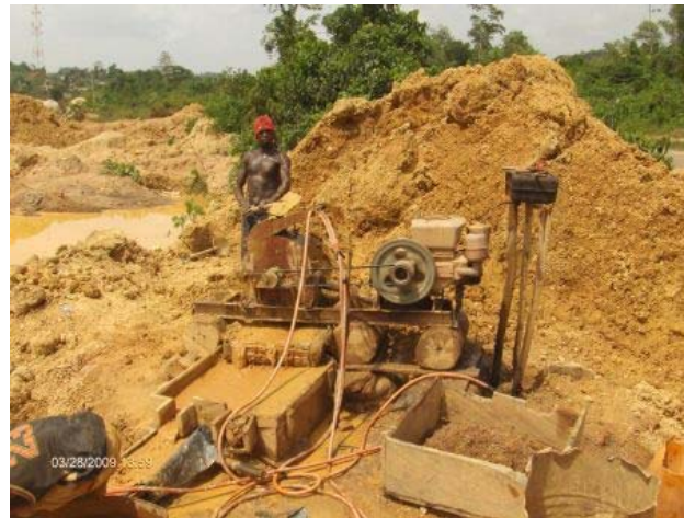
Figure 9. Dozens of washing machines such as this Chinese Chang Fa type are deployed. This machine was working less than 10 m from the road.
