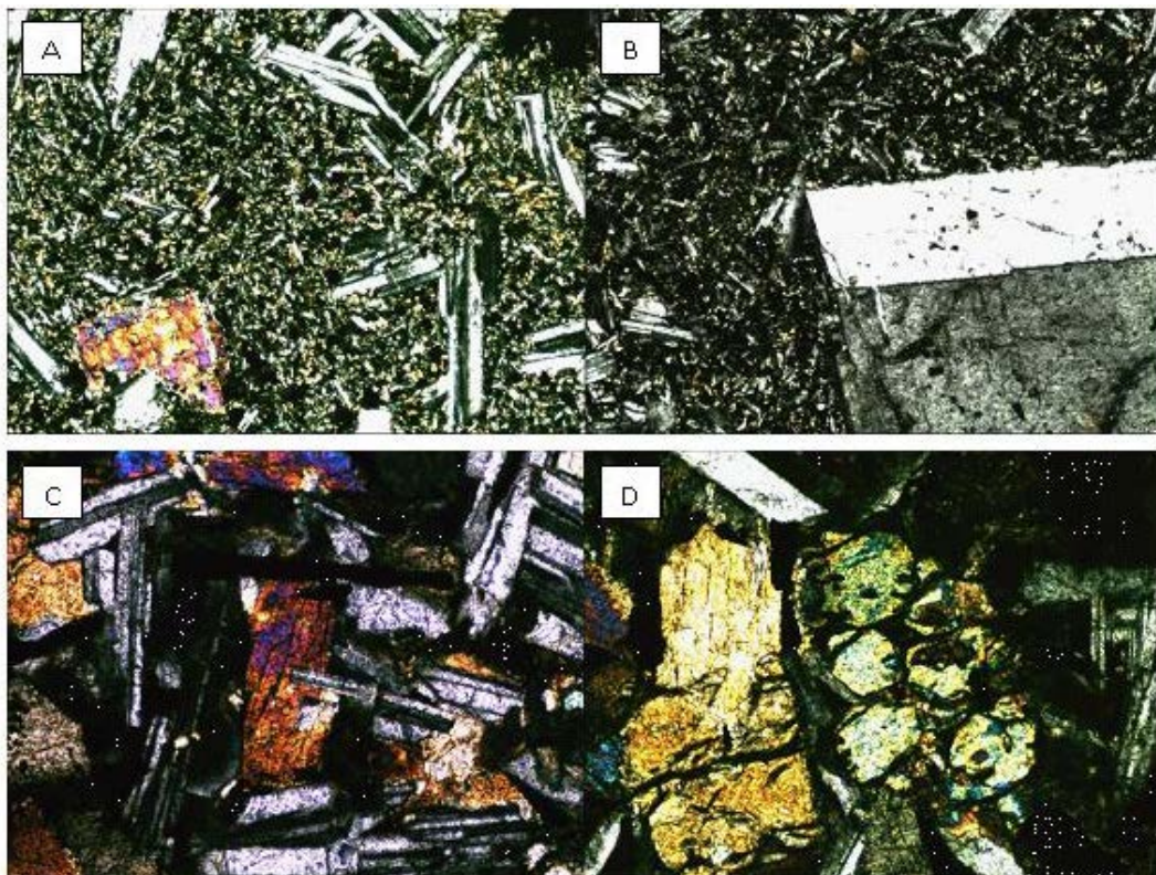
Figure 4. Photomicrographs of QMD basalt showing different textures: (A) Porphyritic and glomerophyritic textures with plagioclase and clinopyroxene (at the left bottom) phenocrysts, and groundmass of plagioclase, pyroxene and opaques, (20×), (XPL); (B) Porphyritic texture with medium size twinned plagioclase phenocryst with inclusions, (50×), (XPL). Sample QD-2; (C) Subophitic texture of pyroxene oikocryst intruded by plagioclase. Iron oxides occur as elongated anhedral crystal that crosscut pyroxene and plagioclase, (100×), (XPL). Sample QD-3; (D) Partly altered olivine crystal. Olivine is fractured and corroded. Iron oxides and opaques fill interstitial between crystals and they crosscut olivine and pyroxene (to the left), (100×), (XPL). Sample QD-3.
