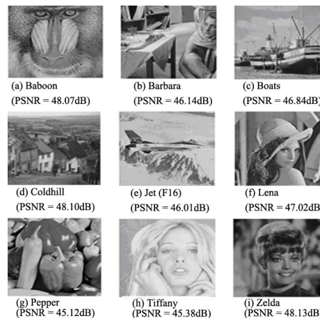
Figure 6. The visual quality of the stego images generated by HClH algorithm with ER = 0.75 (bpp).
