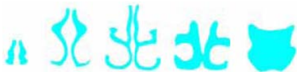
Figure 4. Sectional pattern of nasal cavity model at 2, 4, 6, 8 and 10 cm along the direction of sound waves.
