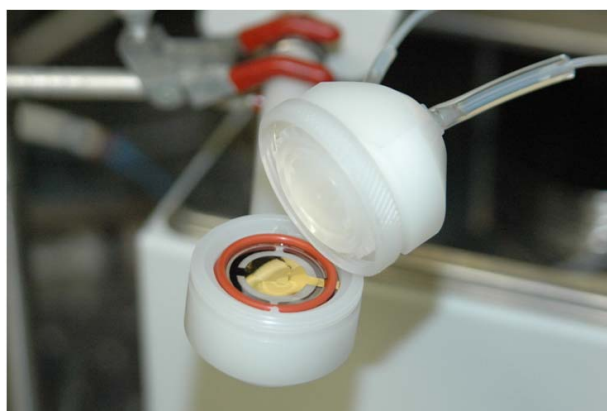
Figure 1. The quartz crystal microbalance (QCM) system. (a) Diagram of the system showing the controller box, the crystal housing, the temperature controlled water bath and the syringe pump and valve switching assembly; (b) Enlarged image of the flow cell with the gold-plated quartz crystal.
