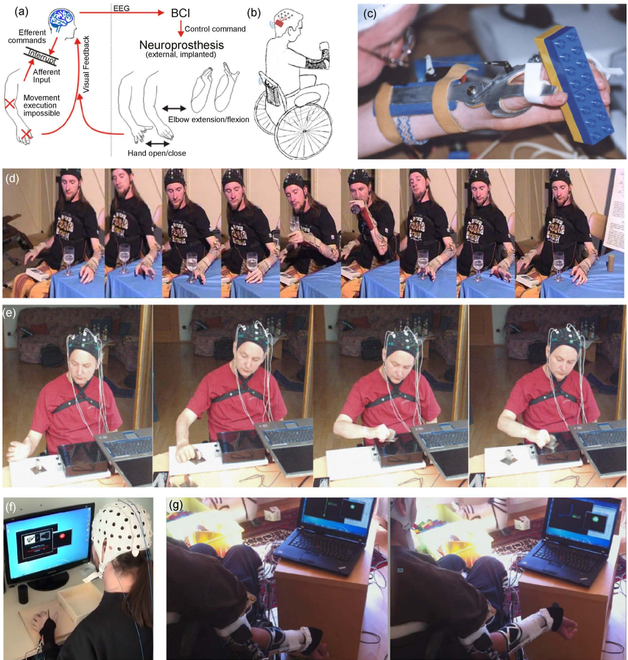
Figure 1. (a) General idea of bypassing the interrupted pathways in the spinal cord with the help of a BCI and motor neuroprosthetics to restore hand and arm function by decoding of motor intentions. (b) Vision of the Graz BCI group: a non-invasive BCI-controlled motor neuroprosthesis. (c) Electrical hand orthosis controlled with a single switch BCI [11]. (d) BCI controls non-invasive grasp neuroprosthesis by stepwise activating different grasp phases. (e) BCI in the control of an implanted neuroprosthesis by stepwise activating different grasp phases. (f) Hybrid BCI to select type of grasp and breaks of stimulation, shoulder position sensor controls stimulation strength and therefore grasp forces. (g) Temporal coding of single motor imagery pattern for the control of hand (open, close) and elbow function (flexion, extension) with the help of a hybrid neuroprosthesis.
