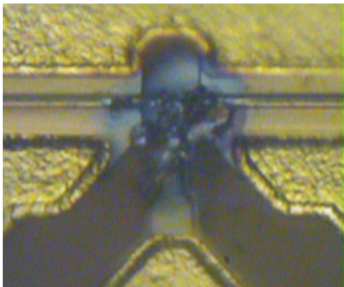
Figure 9. Micrograph of LNA damaged
