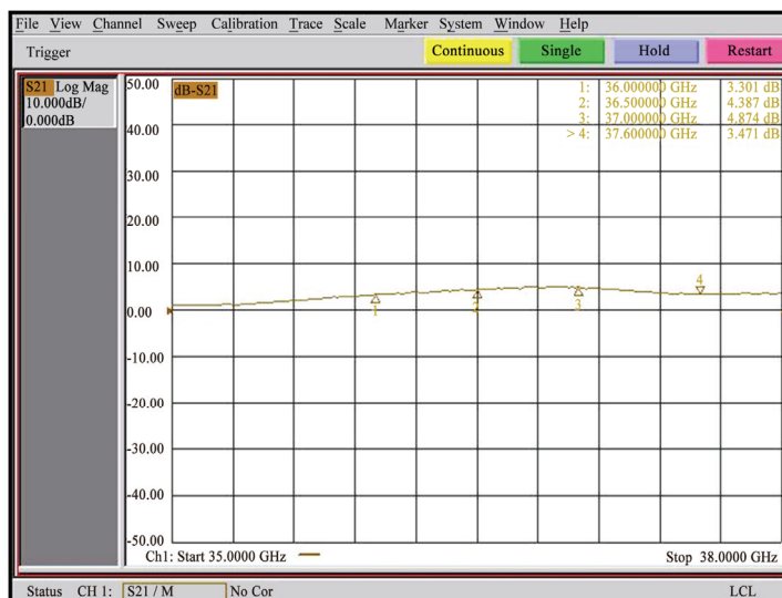
Figure 6. The gain of LNA after experiment
