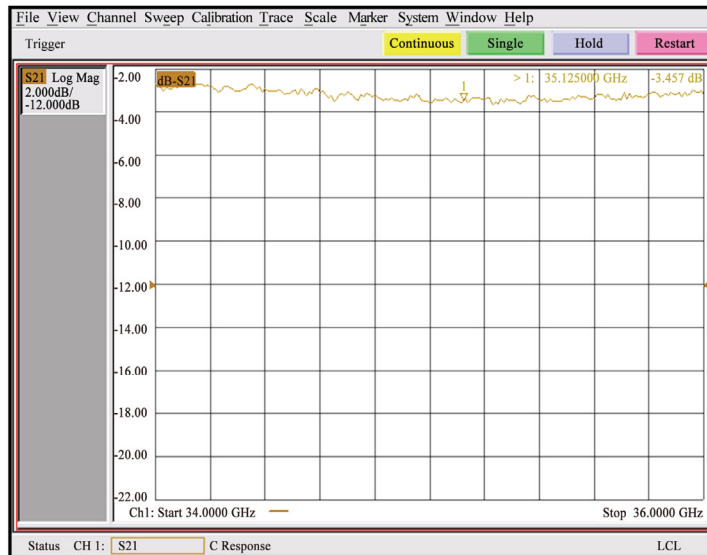
Figure 7. The insertion loss of Limiter before experiment
