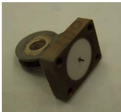
Figure 10. Photo of the input and output antenna assembly.
