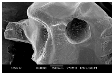
Fig (b) Micro cavity present
