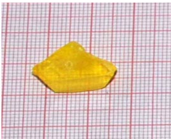
Figure 4. Photograph of as grown crystal of PNPIB by slow evaporation method.
