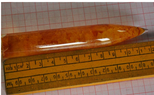
Figure 5. Photograph of as grown PNPIB single crystal by S-R method.
