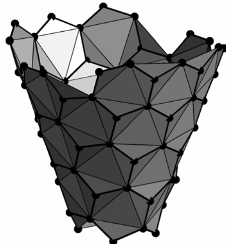
Figure 13. The polyhedric model of a nanocone \delta = 38.94^\circ .
