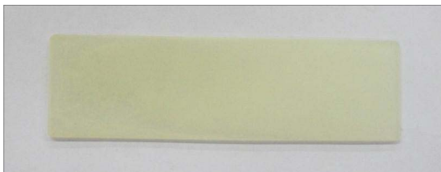
Figure 2. A photo of spray pyrolyzed ZnO nanofilm on glass samples.
