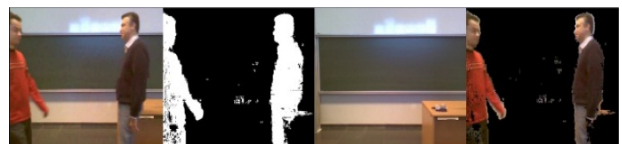
Figure 4. Foreground subtraction results for a particular frame in a video sequence.
