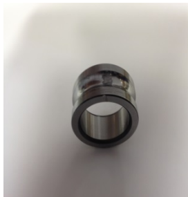
Figure 4. Inner race fault.
