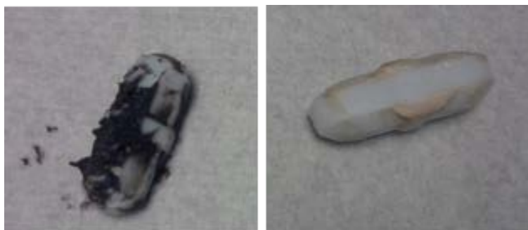
Figure 9. Appearance of stir bars from a mixture of Z-TiO 2 and naphthenic acid (Right) after exposure to UV light for 5 days and (Left) kept in dark for a week.
