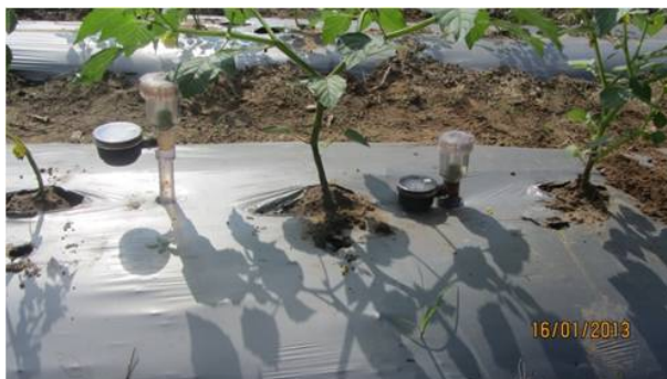
Figure 2. Monitoring soil moisture tension at two depths (15 and 30 cm) in husk tomato cultivation.
