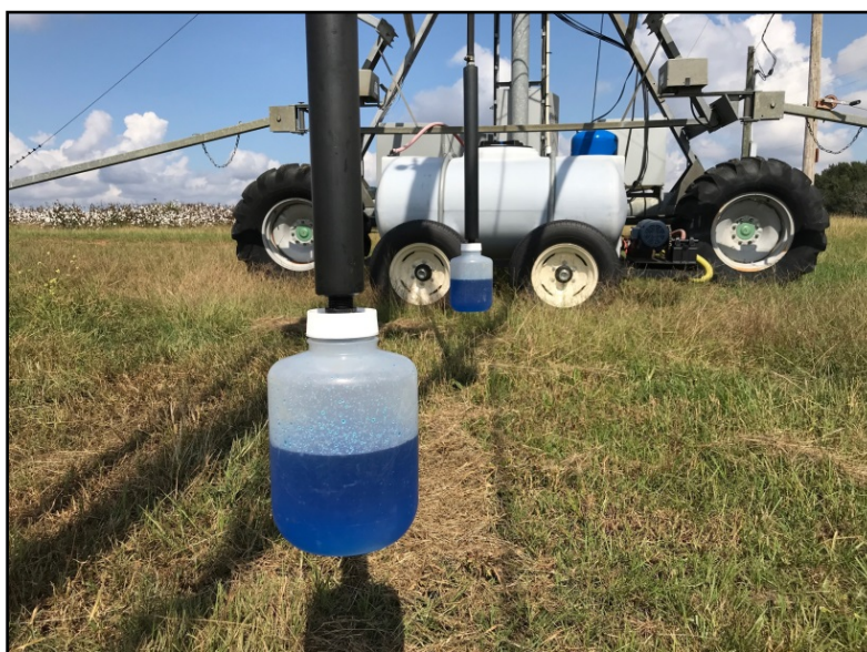
Figure 6. A 3-L calibration bottle connected to the end of the LEPA irrigation drop hose.
