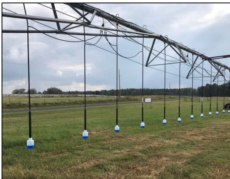
Figure 8. Uniformity test sample collection using 3-L bottles attached to the LEPA drop nozzles.
