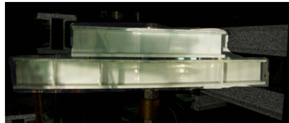
Figure 5. Combination beams loading method.
