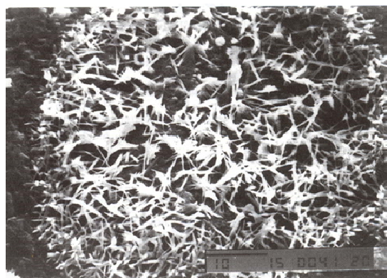
Figure 4. SEM photomicrograph showing the formation of a protective film of boehmite on alloy 4. The needle shaped structure is seen on the alloy surfaces.
