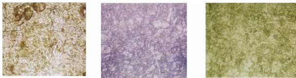
Figure 1. Present the microstructure of 9% Ni steel plate.
