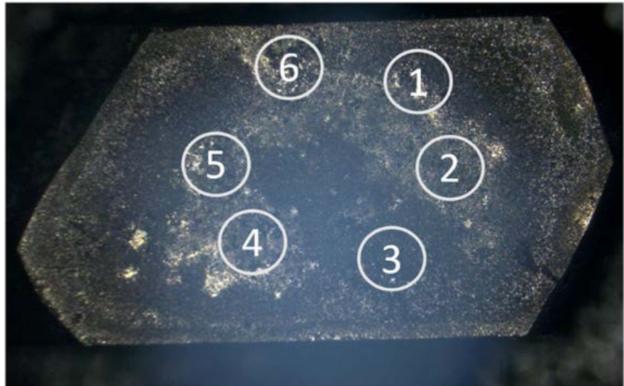
Figure 3. Appearance of the modified surface and the hexagonal spots showing the magnet formation.
