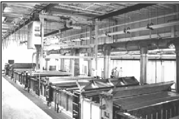
Figure 3. Overview of the bath of nickel-phosphorus.
