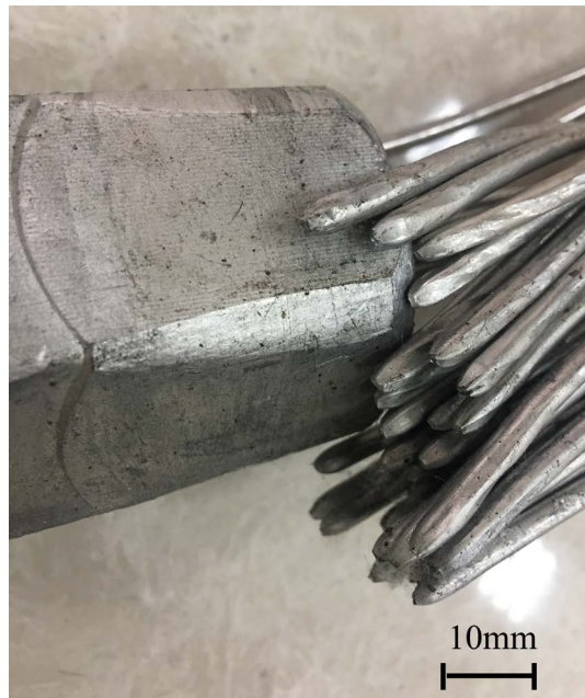
Figure 6. The fracture surface morphologies of the fractured aluminum strands after mechanical test.
