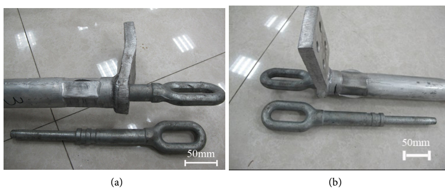
Figure 5. (a) The aluminum tube crimping into different locations of the steel anchor (a) on the grooves (b) on the polished rod.
