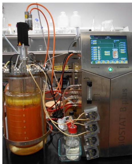
Figure 3. Mass production of H. bacteriophora in a 10 L bioreactor. Note the red pigmentation produced by its bacterial symbiont P. luminescens .
