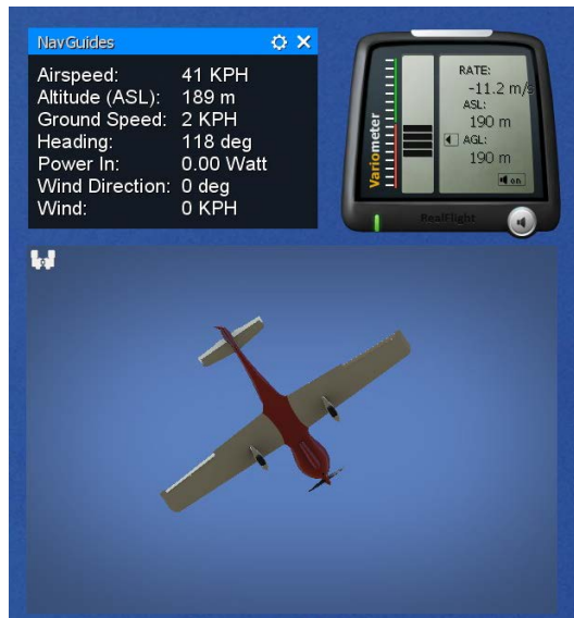
Figure 2. Dynamic parachuting: stall-spin maneuver performed by the SP-1 with the variometer showing a descent rate of 11.2 \text{ m}\cdot\text{s}^{-1} . Full deflection of the control surfaces can also be observed.
