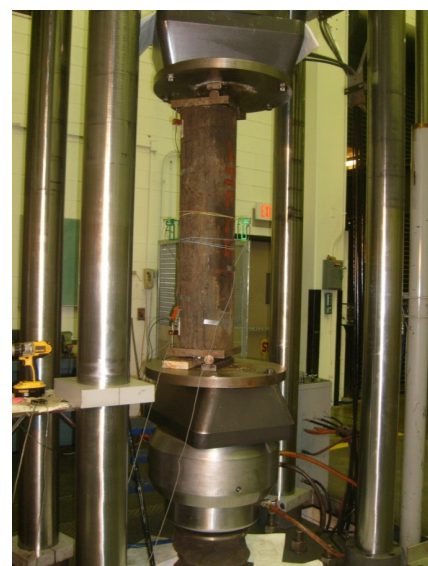
Figure 11. Installed specimen in the MTS testing machine.
