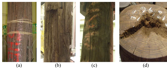
Figure 4. Different types of decay observed in the tested pile specimens: (a) Vertical crack; (b) Partially crushed fibers; (c) Irregular shape; (d) Mold and fungus inside of cracks.
