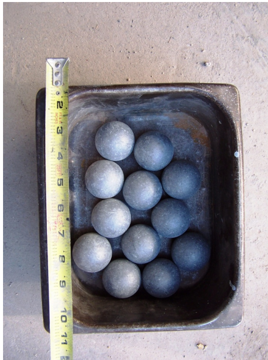
Figure 3. Steel spheres used in LA Abrasion steel cage.
