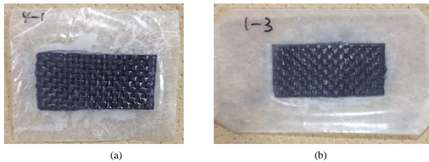
Figure 13. Typical specimen configuration after curing (degree of cure of 0.68). (a) Specimen with electrical short; (b) Specimen with capacitance.
