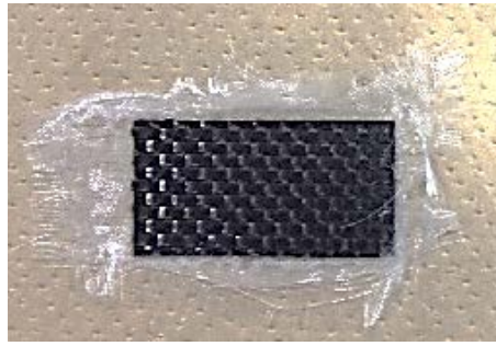
Figure 2. Typical example of structural capacitor specimen.
