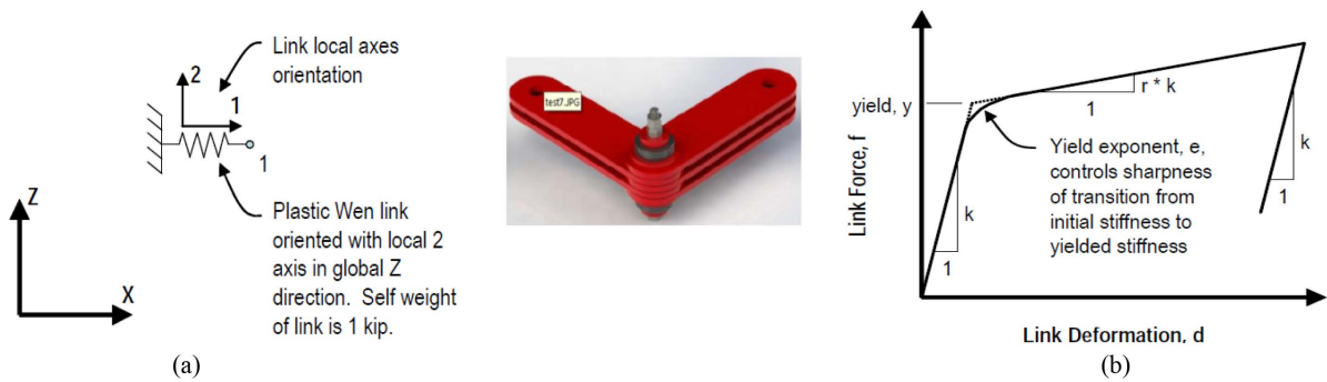
Figure 12. (a) The power relationship-transmission of the damper (FD); (b) The form and damper model [14].
