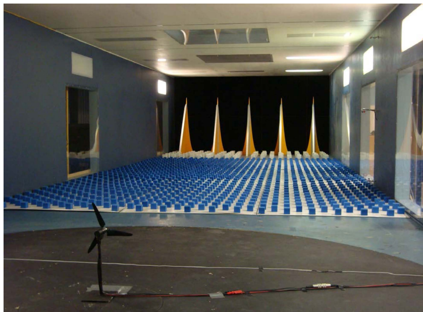
Figure 2. Picture of the wind tunnel looking upstream with the turbine model and the roughness elements and spires used to create the atmospheric boundary layer.
