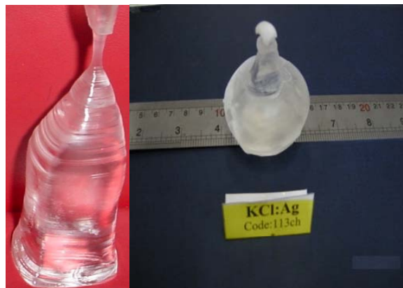
Figure 2. The single crystals KCl:Ag and KCl:In after exit of the furnace.
