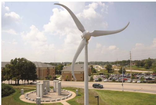
Figure 1. Skystream3.7 wind turbine used for experimental validation.
