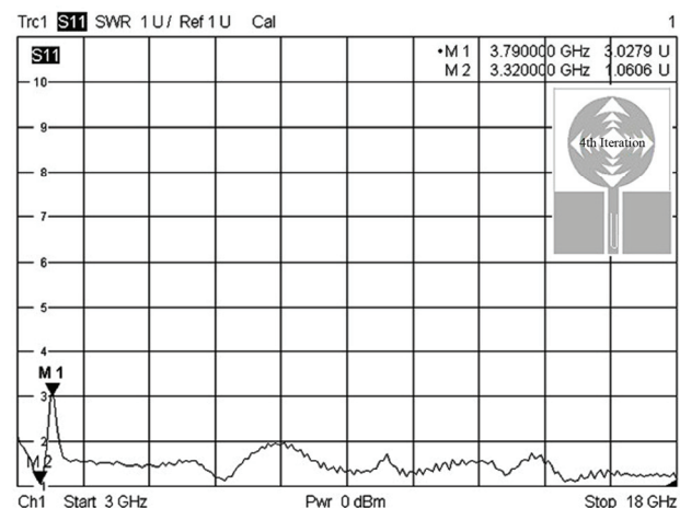
Figure 13. Experimental VSWR of circular fractal antenna with U-type slot.
