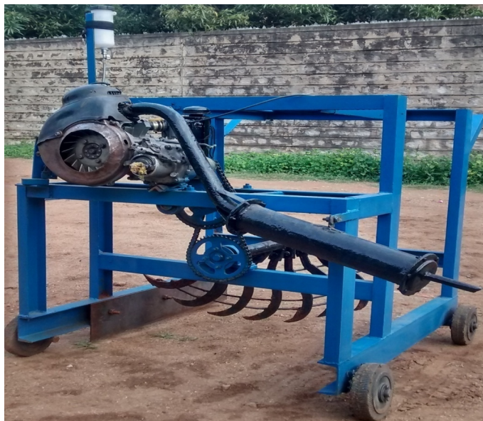
Figure 14. Fully assembled ginger harvesting machine.
