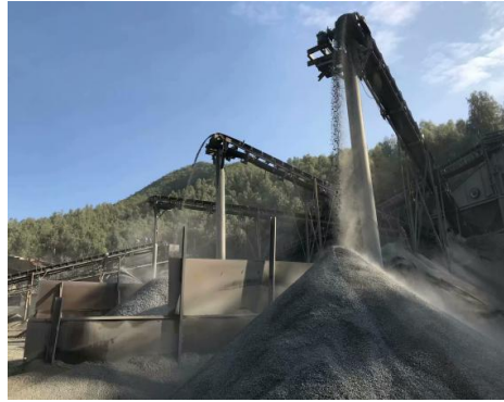
Figure 3. Machine-made sand processing.
