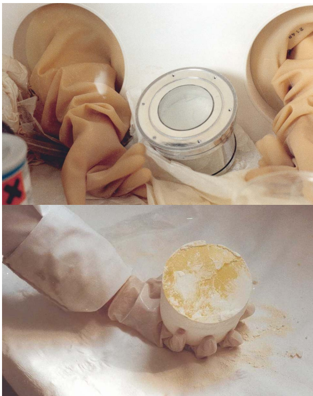
Figure 13. NaI (Tl), out of his casing and humid has lost its transparency. After chemical treatment in a dried glove-box and re-encapsulation in its casing, the transparency and measurement qualities are recovered.
