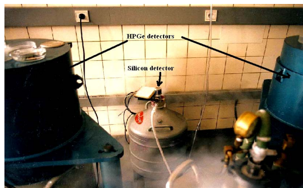
Figure 12. Silicon diode for the measurement of low energy gammas from samples used outside a shielding room.
