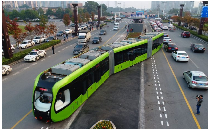
Figure 4. The trackless tram system by CRRC and demonstrated in Zhuzhou, China.
