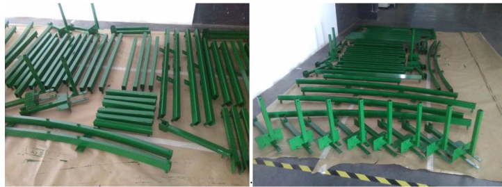
Figure 20. Platform parts before mounting.
