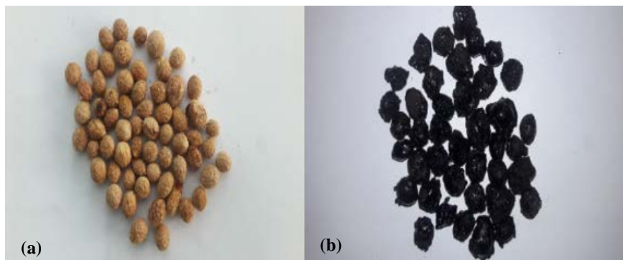
Figure 2. (a) Jujube seeds before the coating operation; (b) Jujube seeds after the coating operation.
