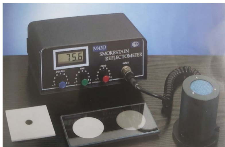
Figure 2. EEL 43M Smoke Stain Reflectometer developed in conjunction with DTI Warren Spring Laboratory.
