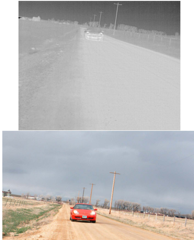
Figure 21. Thermal and corresponding RGB images of field test at 100 ft.
