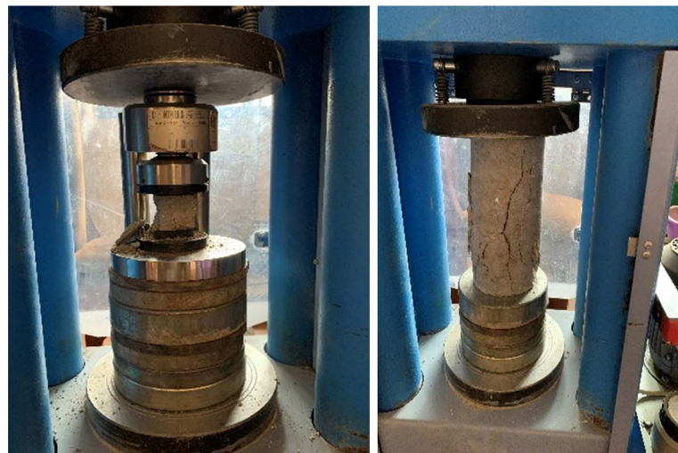
Figure 3. Compression tests on Mortar and concrete specimens.
