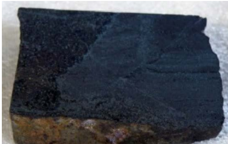
Figure 12. TG-5 Magnetite hematite ore.
