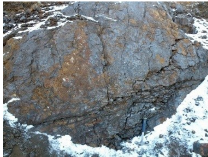
Figure 3. Strong magnetic sulphide containing magnetite ore.
