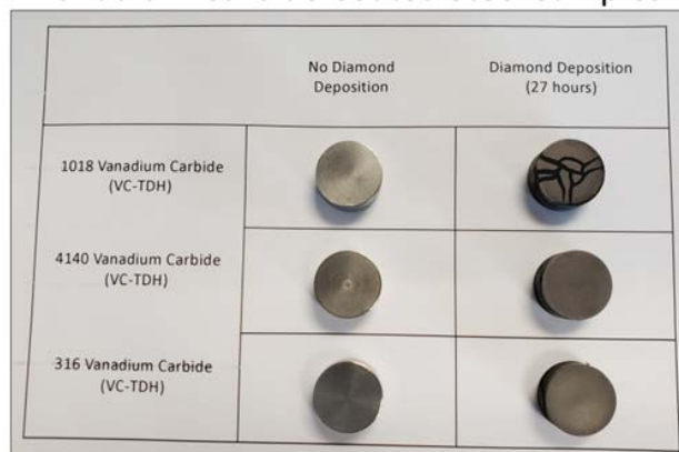
Figure A3. Layout of diamond-coated steel samples with VC interlayer.
