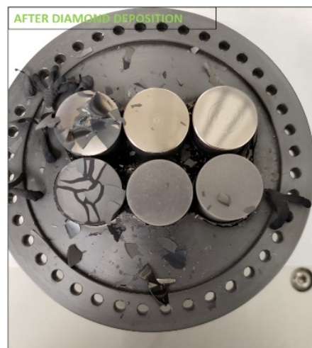
Figure A2. VCN (top and VC (bottom) coated steel alloys after long MPVCVD diamond deposition.
