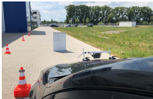
Figure 8. Measurement setup to determine the radar cross section of physical test objects.
