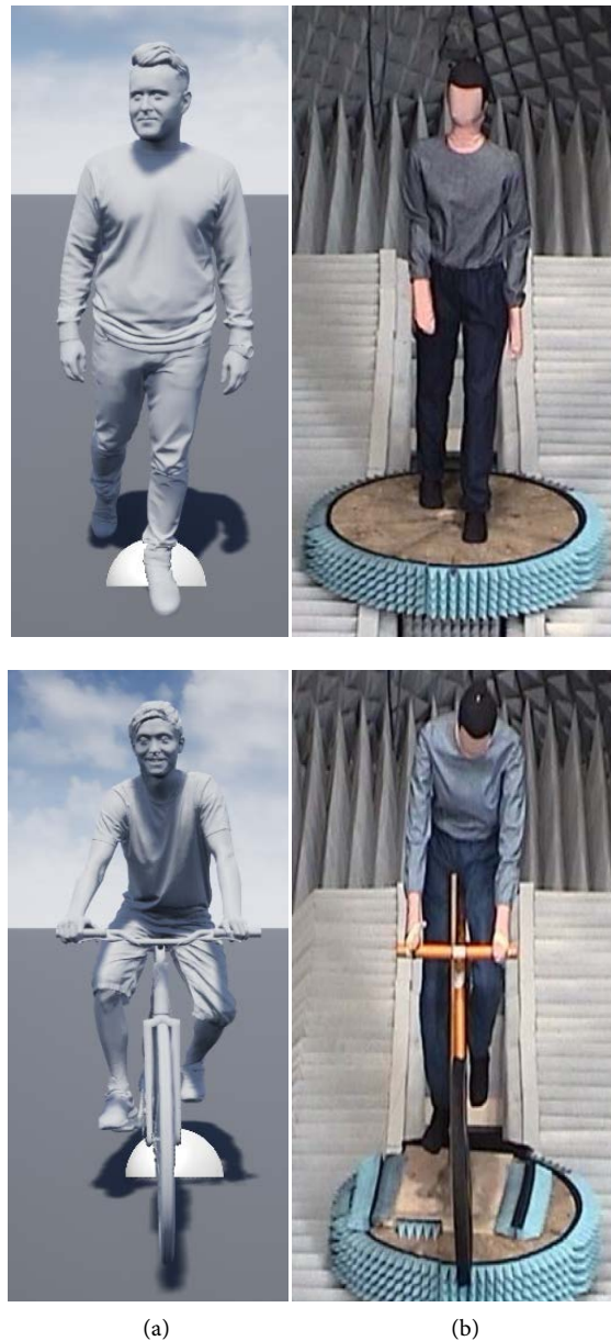
Figure 10. Selected models for the comparison of measured radar signatures with simulated results; (a) Used virtual 3D-models; (b) Measured Models from [13].
