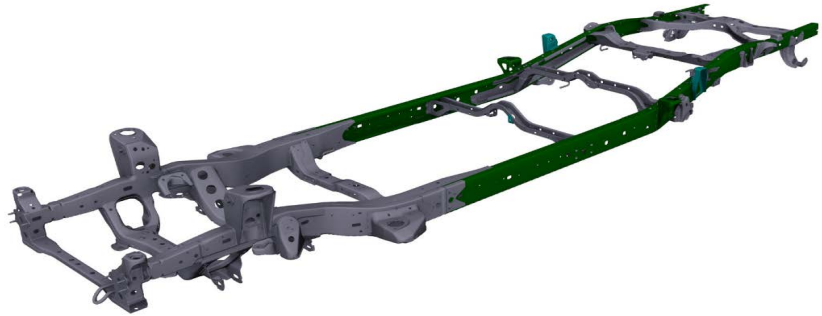
Figure 1. Original truck frame configurations.
